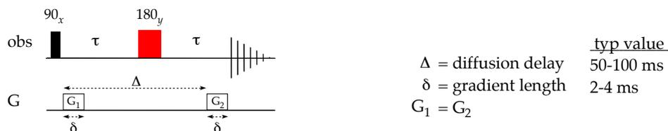
The peak attenuation is controlled by three variables. Typically, the gradient power ( $G$ ) is varied over the course of the 2D experiment. The diffusion delay ( $\Delta$ ) and gradient length ( $\delta$ ), however, must be optimized.
