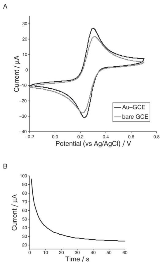
Figure 3. (A) Cyclic voltammograms of bare GCE and Au-modified GCE in  $0.002$  M potassium hexacyanoferrate(III) at  $100$  mV s<sup>-1</sup>. (B) Electrochemical signal recorded during the electrodeposition of gold nanoparticles onto the GCE.
